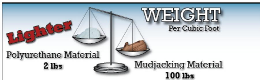
Mudjacking uses a grout based material infused with mud and Portland cement. It is hydraulically pumped under the concrete to fill in voids and raise the concrete. Foam jacking uses a polyurethane foam material that
